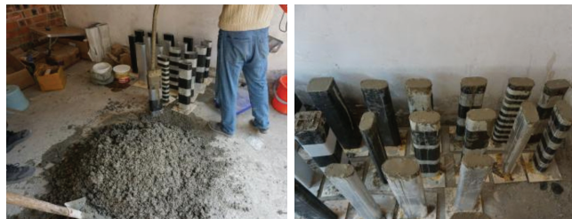
(a) 试件浇筑 (b) 试件养护
