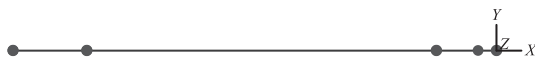
图 9 计算段弹性地基梁模型 Fig. 9 Beam model of elastic foundation in calculation section
