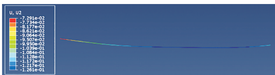
图 11 计算段轴线沉降云图 Fig. 11 Settlement nebulae of calculation section axis
