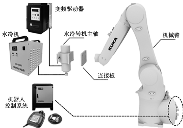
图2 建造装备系统 Fig.2 Construction equipment system
